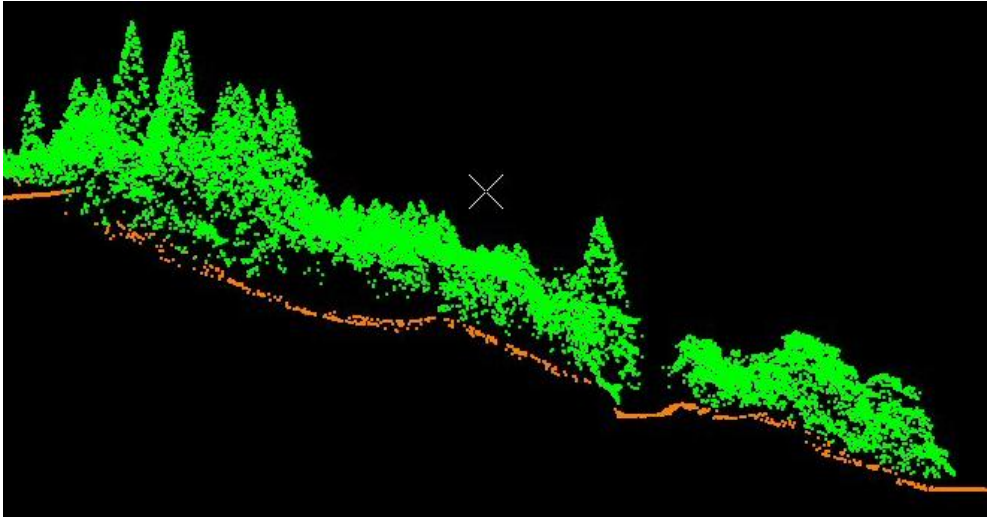
11 12 Fig. 5. Vegetation distribution and structure shown by classification of an airborne lidar 13 point cloud. Data illustrated were provided courtesy of Forest Research, UK. Location: 14 Scottish Highlands, UK.
