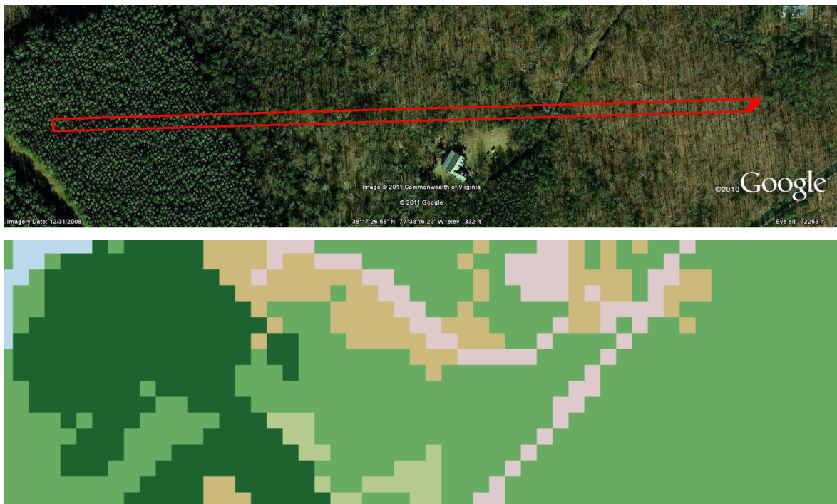
Figure 1. Test site near Fredericksburg, Virginia, USA. Above: GoogleMaps image with a 800m section outlined in red; Below: National Land Cover Data (US Geological Survey). Mid green represents deciduous forest; evergreen forest is indicated in darker green, light green is mixed forest, pale pink is developed/open space, and beige is shrub/scrub. Some misclassification can be observed which would have implications for biomass mapping using this dataset for stratification of the landscape.
